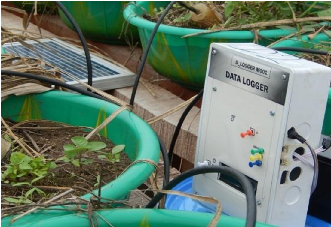
Plate 3: Fabricated data logger for monitoring soil water content
