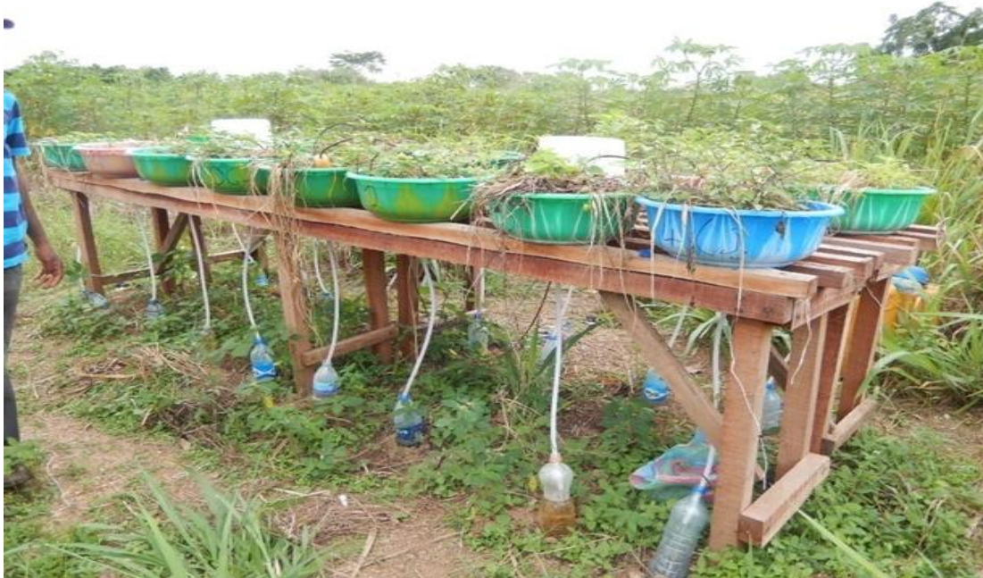
Plate 4: Setup of lysimeter instrumented with fabricated datalogging TDR soil water sensor
