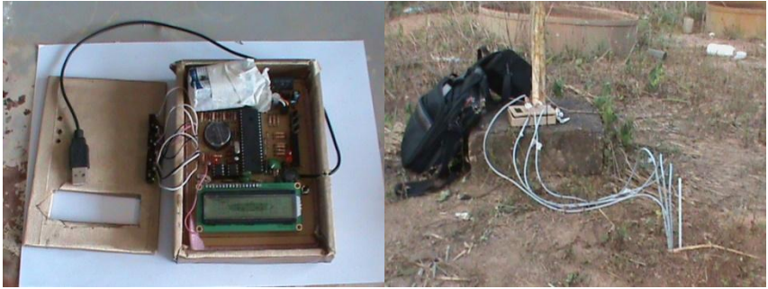
Plate 2: Fabricated datalogger and the TDR water sensor installed in the soil
