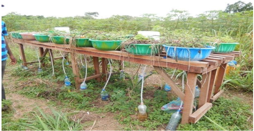
Plate 4: Setup of lysimeter instrumented with fabricated datalogging TDR soil water sensor
