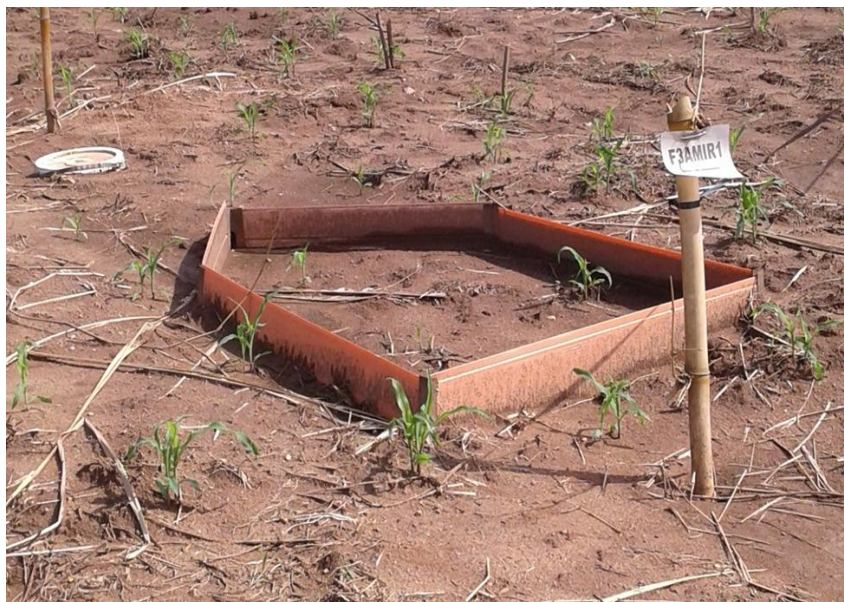
Plate 11: PVC bounded runoff plot installed on the field to harvest runoff and sediment loss into a 25 litre bucket
